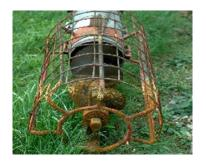
5. Auger has a properly designed intake guard in place that is in good condition.
