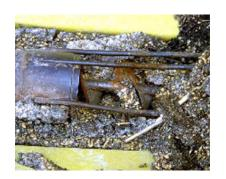
3. Auger has a properly designed intake guard in place but it is bent or damaged; auger has an improperly designed intake guard.
